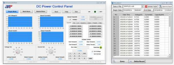
When the communication port has more than one power supply connection, it enters the Multi Mode interface. Supports switching control or display current power supply's settings.
